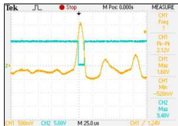
Figure 6. The signals observed at TP1(orange) and TP2(cyan) when the charged particle was detected.
