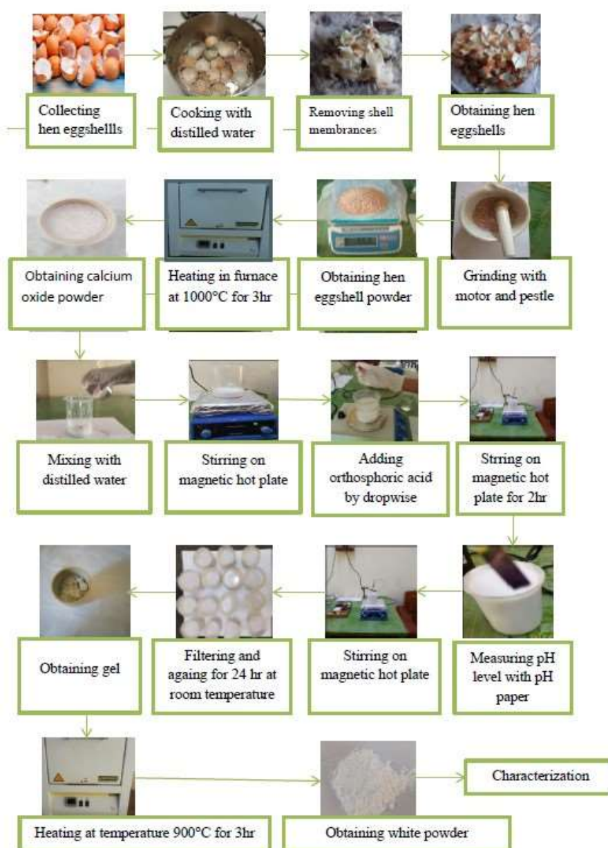
Figure 1. The sample preparation of hydroxyapatite powder from hen eggshells by precipitation method
